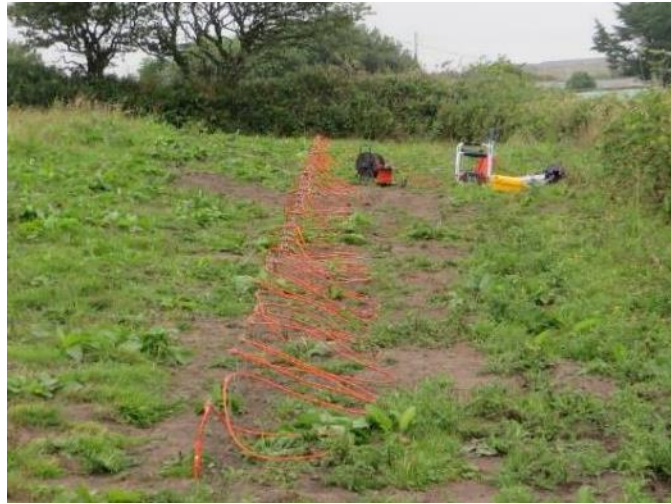
Figure 2.9 The resistivity line of electrodes at the lower end of daffodil field 2
