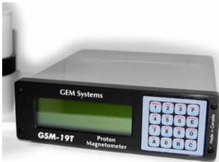
Figure 5-22 The data logger part of the GSM-19 system (GEM 2008).
