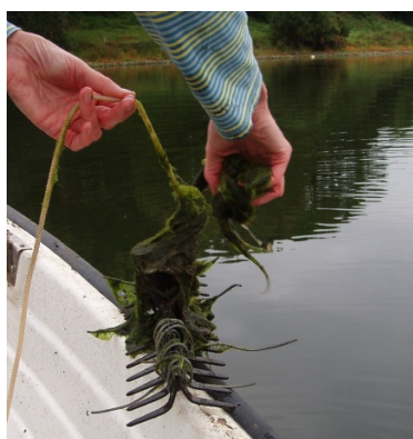
Grapnel: Two rake heads wired together and attached to a line
