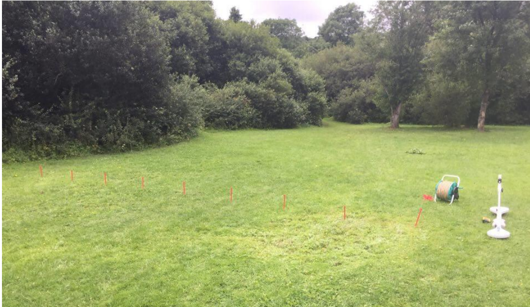
Figure 16 Photograph illustrating the grid system used to collect the EM data. The red stakes mark the start and end of each transect line. Source: Author, 2016
