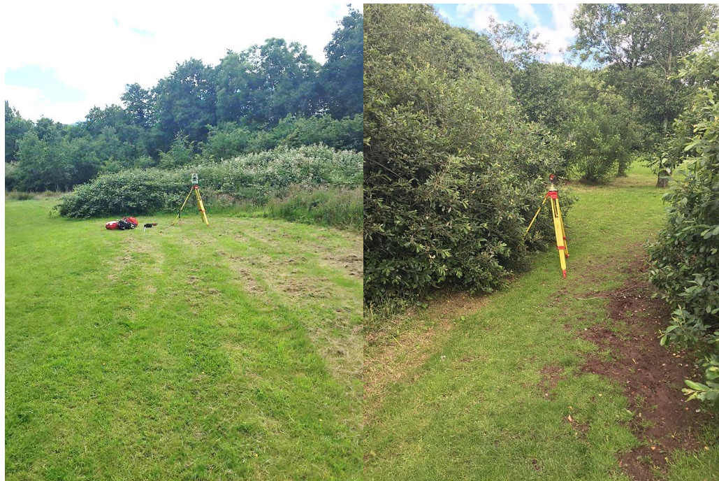
Figure 11 photographs of the temporary station traverse around Area 4 on the Penrose amenity site. Source: Author, 2016.
