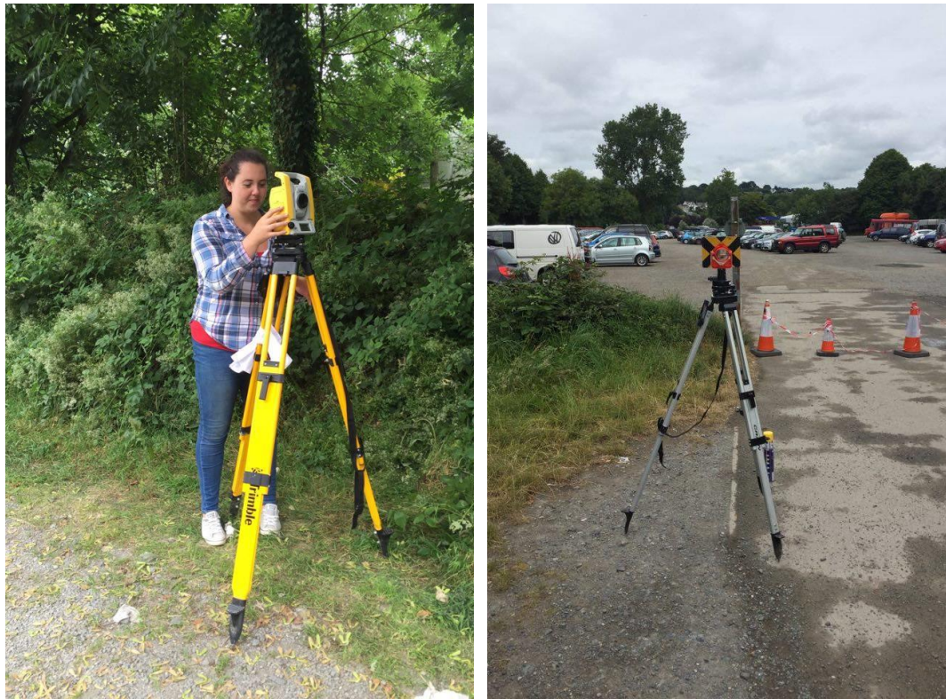
Figure 13 Photographs of the resection setup to survey the positions of each electrode used for Electrical Resistivity.
