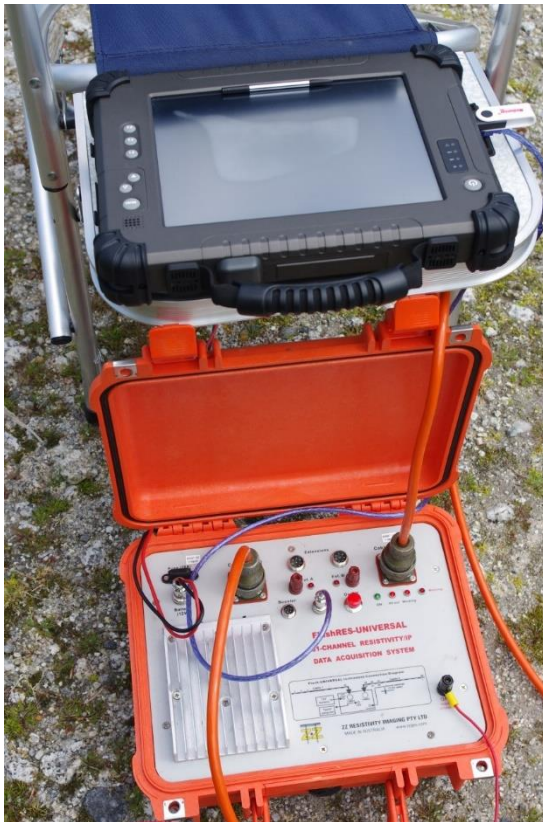
Figure 12 Photograph of the FlashRES-Universal 96 system used for the resistivity data collection, it also shows the laptop used to run the data acquisition. Source: (N. Wood, 2016).
