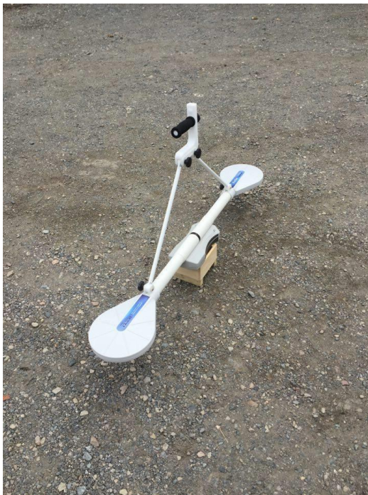
Figure 14 Photograph of the EMP-400 Profiler in the field (Source: Author, 2016)
