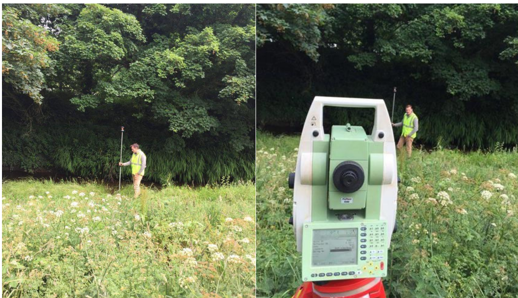
Figure 10 Photographs of detailing the top of the river bank at Penrose, Helston. Using a detailing pole and 360 Prism. Source: Author, 2016.
