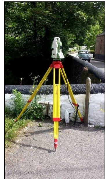
Figure 5:3- Leica 1200 Total Station setup and levelled over control station- Pavement, in order to setup using the known back sight function. (Source: Authors own.)
