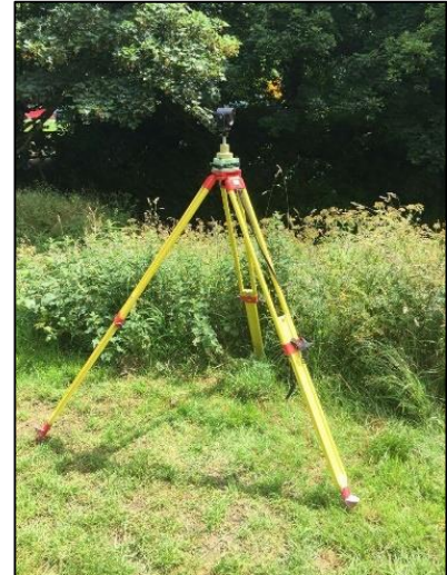
Figure 5:2- Tripod and Leica Circular Prism set up (centred and levelled) over the control station Bridge, for use in resection. (Source: Authors Own.)
