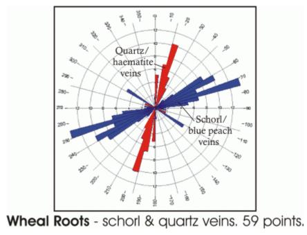
Figure 6. A rose diagram of lode and vein orientations at Wheal Roots.
