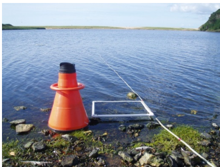
Photo 6: Permanent transect survey equipment: Bathyscope, quadrat and weighted rope (Jan Dinsdale)
