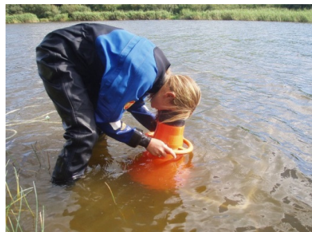
Photo 7: Surveying with bathyscope. Wearing a dry suit 0.5m was very useful when surveying the deep end of the transect (Jan Dinsdale)
