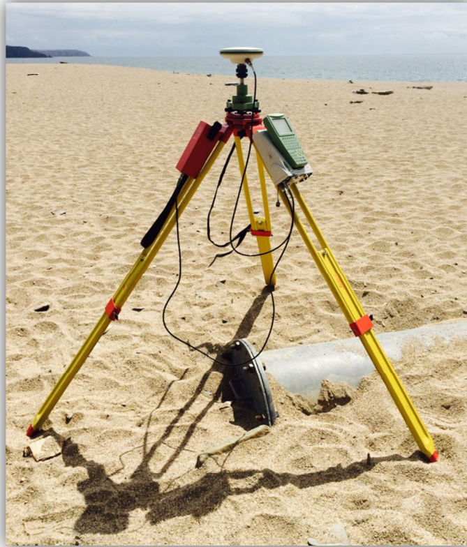
Figure 44: Photograph of the GPS station set up over a point marked on the pipe to create another base station for future resection use.
