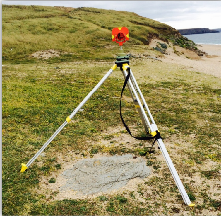
Figure 39: Leica prism set up on a tripod over base SE, used in resection.
