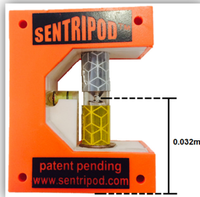
Figure 41: Photograph of a Sentripod. Height of target is marked (not to scale).
