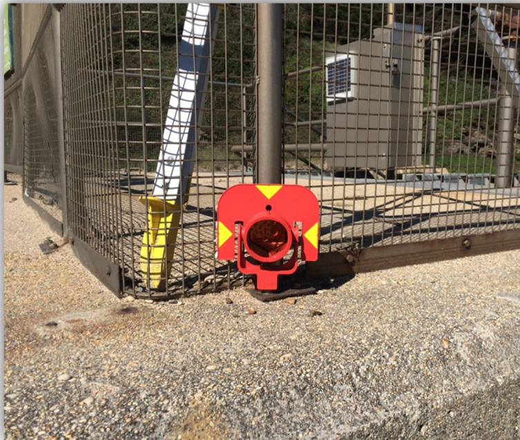
Figure 53: Circular prism placed on the bolt for determining coordinates. Note the collar to the right of the prism which obstructs the view to the sentripod from certain places on the bar.
