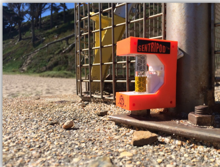
Figure 55: Sentrypod placed on bolt a held level and in place using tac. This can be used in resection if view of Base NW is obstructed. Note the sentripod fits over the 5mm tall bolt, providing the need to adjust the target height to 0.027 rather than 0.032.
